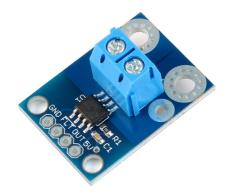
This board carries the Allegro's ACS711ELCTR-12B-T hall effect-based linear current sensor, which offers a low-resistance ( $\sim$ 1.2m $\Omega$ ) current path.
